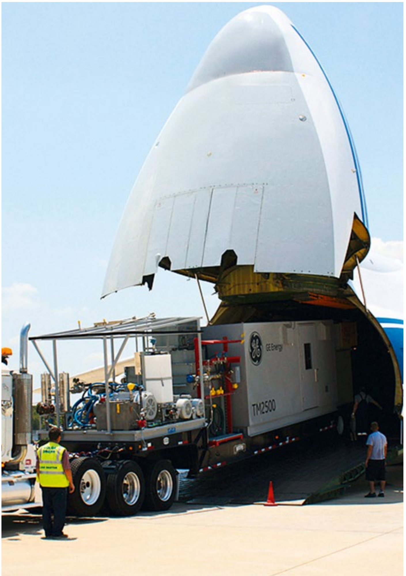
GE's trailer-mounted TM2500* aeroderivative gas turbines can be moved quickly and installed in days.
