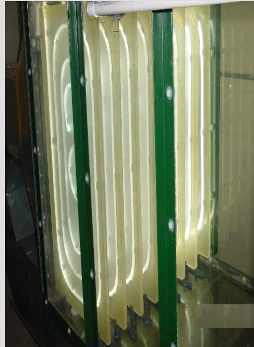
Lighting panels viewed from direction of gas flow
